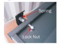
Slide spring on the shaft of the stabilizer. Push the shaft thru the hole of the panel. Secure lock nut. Make sure you see 2 to 3 full threads.
